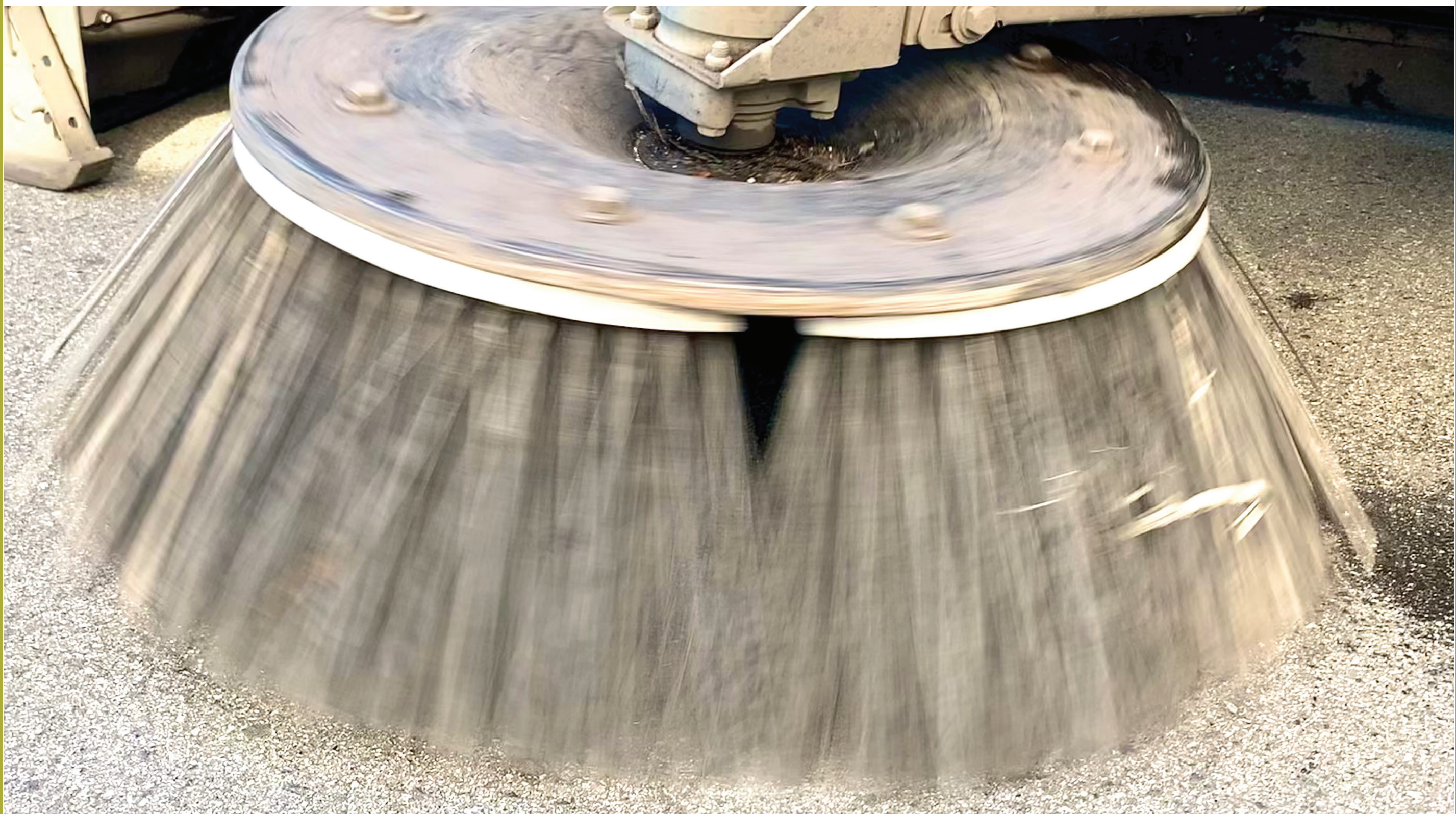
The rotating gutter brooms on mechanical sweepers dislodge debris from the pavement and then a vacuum in the truck sucks up the rubbish and leaves.
