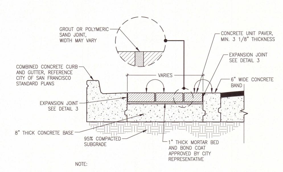
1. MORTAR SHALL CURE FOR 72 HOURS MINIMUM BEFORE ALLOWING VEHICULAR TRAFFIC UNLESS OTHERWISE APPROVED BY CITY REPRESENTATIVE.
