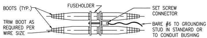
**2-POLE SIMULTANEOUS DISCONNECTING WATERPROOF FUSEHOLDER**
