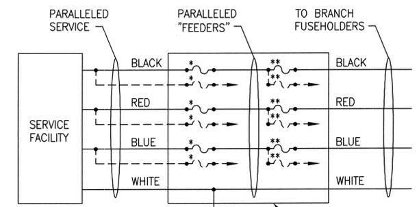
NOTE: PARALLELED 'MAIN' FUSED CONNECTORS REQUIRED FOR SERVICES OVER 70 AMP. ON FUSE HOLDER REQUIRED FOR EACH #8 & #6 'FEEDER'
