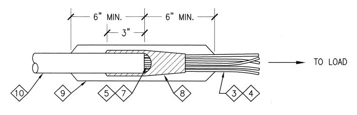
NOTE: BEFORE INSTALLING COMPOUND, PROVIDE 1/8" SPACING BETWEEN EACH CONDUCTOR TO ASURE WATERTIGHT SEAL
