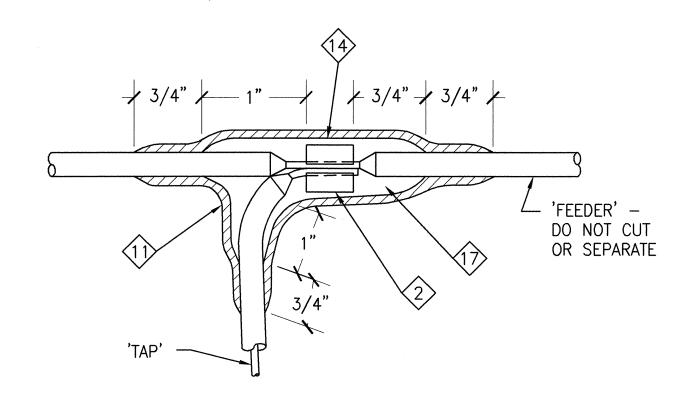
TYPICAL 'TAP' SPLICE FOR SINGLE CONDUCTOR WIRING
