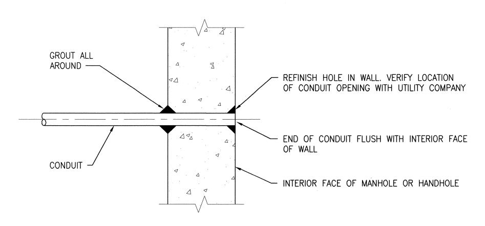
INSTALLATION OF SERVICE CONDUITS IN OR ON UTILITY OWNED WOOD POLES, MANHOLES & HANDHOLES
